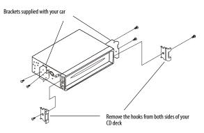
2 Mount the brackets to the sides of the CD deck using two screw holes on each side.
